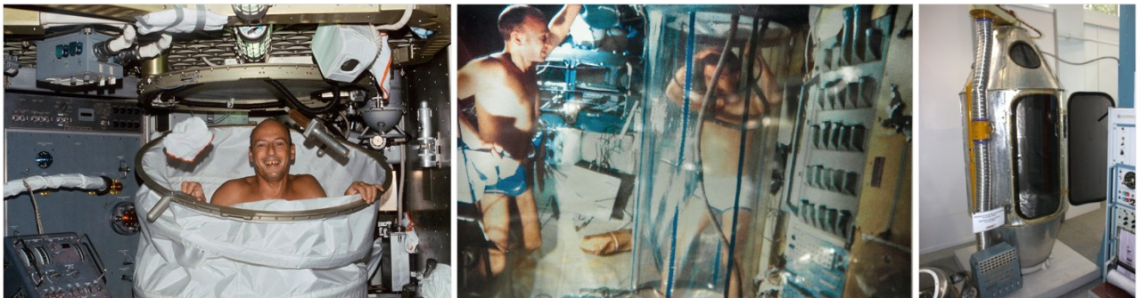
Figure 3. Left to right: NASA’s Skylab space shower, Russian Salyut 7 space shower, MIR Space shower/sauna.
